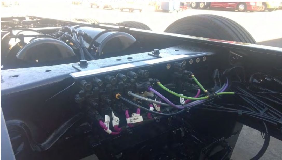
FIGURE 7-45. EOA Solenoid Location for Chassis Built After 1/1/2016
