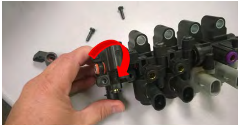
FIGURE 7-48. 23 EOA Solenoid Disassembly
