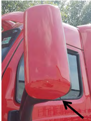
FIGURE 2-3: Aerodynamic Mirror OAT Sensor Location
