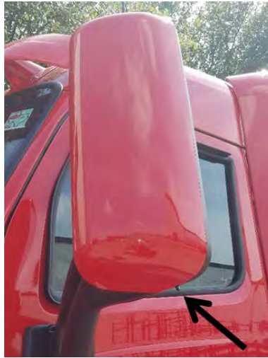
FIGURE 2-3: Aerodynamic Mirror OAT Sensor Location
