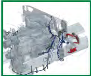
ENGINE HARNESS 1) Connections to Main Chassis Harness 2) Connections to Firewall Bulkhead 3) Connections to Starter 4) Connections to Aftertreatment Harness 5) Connection to Engine ECU
