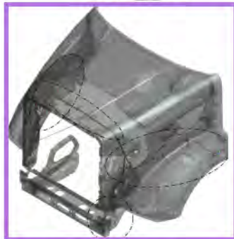
HOOD CHASSIS HARNESS 1) Connections to Main Chassis Harness 2) Connections to Head Lights 3) Connections to Turn Signal Lamps
