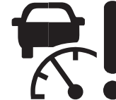
Active Cruise and Braking (ACB) Fault Alert
