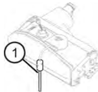
1. DEF Tank Vent
