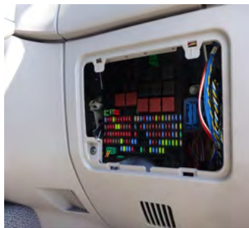
Figure 7-2.2 Inside View - Electrical Junction Box Location
