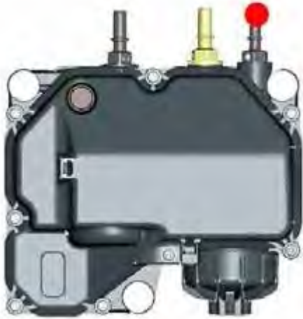
Figure 4-2 Measurement Location of DEF Supply Module (Pump)
