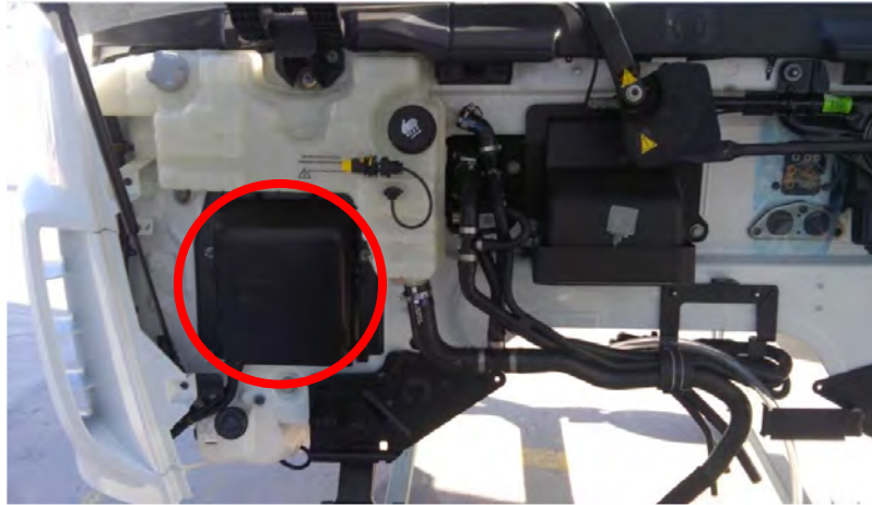
Figure 7-3.1 Electrical Junction Box Location
