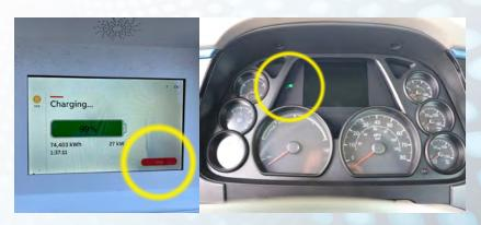
iv. Battery balancing occurs during the last 10% of charging. For the longevity of the battery system make sure to fully charge the truck at least once a week.
