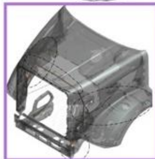
HOOD CHASSIS HARNESS 1) Connections to Main Chassis Harness 2) Connections to Head Lights 3) Connections to Turn Signal Lamps
