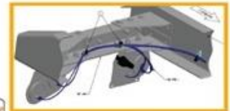
REAR CHASSIS HARNESS 1) Connections to Chassis Harness 2) Connections to Tail Light
