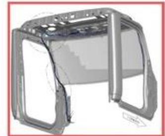
CAB ROOF HARNESS 1) Connections to Main Cab IP Harness 2) Connections to Antennas 3) Connections to Roof Lighting
