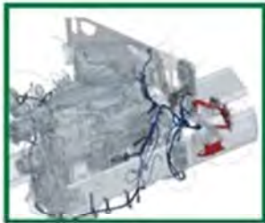
ENGINE HARNESS 1) Connections to Main Chassis Harness 2) Connections to Firewall Bulkhead 3) Connections to Starter 4) Connections to Aftertreatment Harness 5) Connection to Engine ECU
