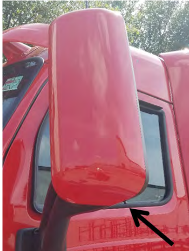
FIGURE 2-3: Aerodynamic Mirror OAT Sensor Location
