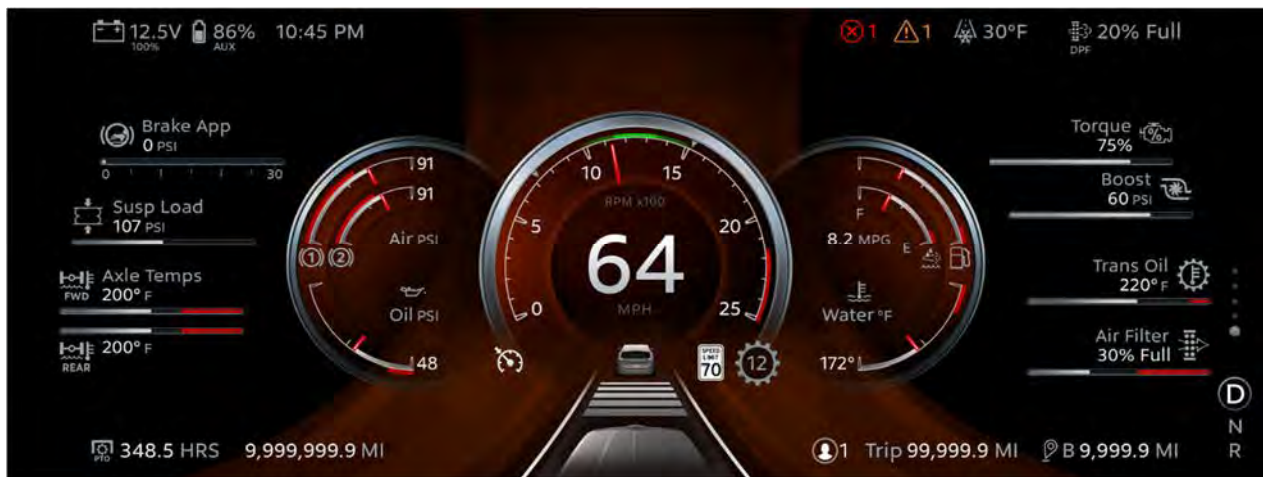
FIGURE 2-4: Digital Display for 579/567.
